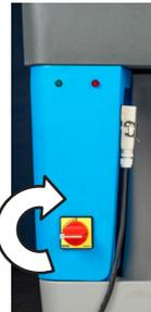
any circumstances and do not use other cleaning liquids unless specifically recommended by the manufacturer. Connect the appliance to the mains with the electrical cable provided. Ensure that the power supply cable is connected to an earth leakage circuit breaker. Switch on the unit by turning the rotary switch to the "I" ON position. Wait for the PLC switch-on cycle, which takes about 5 seconds,
