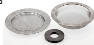
Supplied with two filters and a magnetic filter as standard: a perforated steel plate filter on the worktop that intercepts coarse materials, below, a fine (600 µ) steel filter for finer materials and a magnetic filter that retains ferrous dust and shavings. It is recommended to wash these filters and the magnet weekly. To do this, remove the filters and magnet from the parts washer and wash them with water and apposite fluid.
