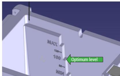
Check the filling level regularly by means of the notches on the wall of the container, as the liquid tends to drop in level due to dispersion and evaporation. If the liquid is below the minimum level, the pump and heater are automatically switched off for safety reasons. Top up the fluid to the optimum filling level, taking care not to exceed the maximum level.
