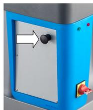
**Attention:** Switch off the pump (by pressing and holding the start button for 1 second) after finishing the washing cycle. However, the unit is equipped with an electronic timer that stops the pump automatically 30 minutes after it has been started. The ti-
