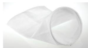
The station is equipped with a 100 µ bag filter positioned under the worktop that collects what may have escaped previous filtering; it has a large capacity but should not be overlooked, as it intercepts the finer particles that accumulate inside it. In this case it is necessary to open the Safe4You table and after locking it with a special rod, the bag filter can be removed and cleaned. Depending on its condition it can be washed or replaced. The standard version has a filter to be replaced.
